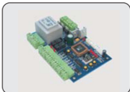
Control board: Intel 80C51 MCU, Controlled silicon Motor control. Parameter
